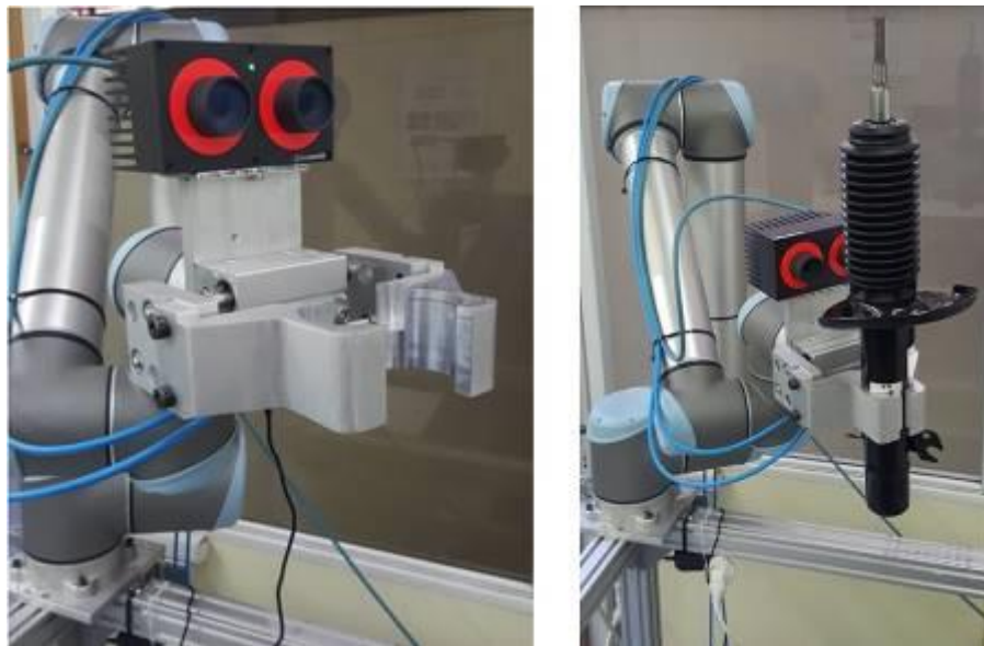
Figure 20. Damper manipulation operations. Left: gripper and fingers. Right: gripper's functionality
